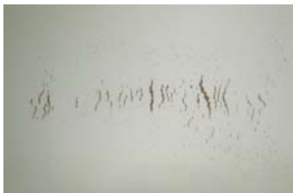
Figure 10. Particulate matter in municipal water supply settled in a bath tub
